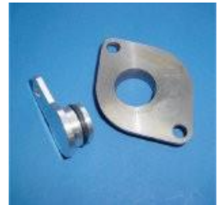
'13-'21 C&C block plug shown with factory freeze plug adapter
