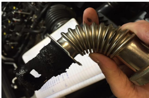
15. Remove EGR bellow pipe(PIC)
